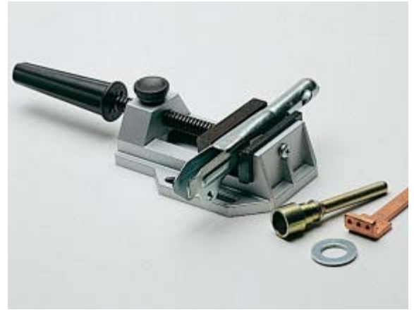
Vice for clamping test specimen; also suitable for mounting on the support plate of measurement stand V18 and V24
