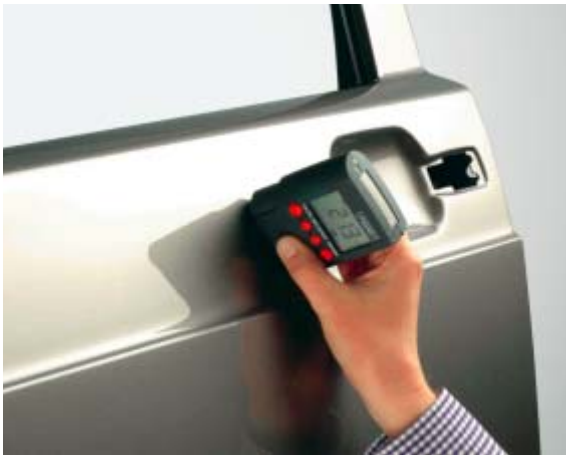
Measurement of the paint thickness on steel sheet using the magnetic induction method
