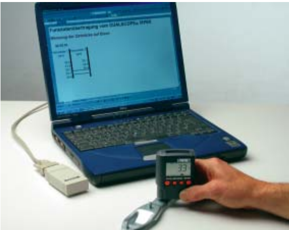
Data transfer via radio (unidirectional)
