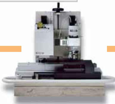
1999 FISCHERSCOPE® H100 C: Newly designed, with improved distance measurement, higher load resolution, integration of XY-control, new software
