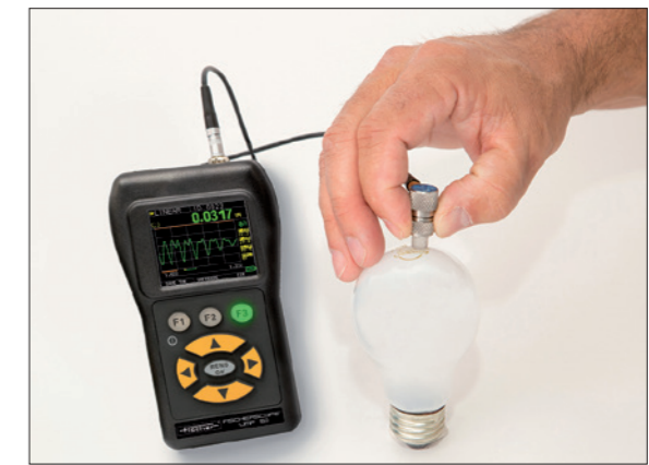
Vibrating alarm and colored LEDs indicate when a threshold has been violated
